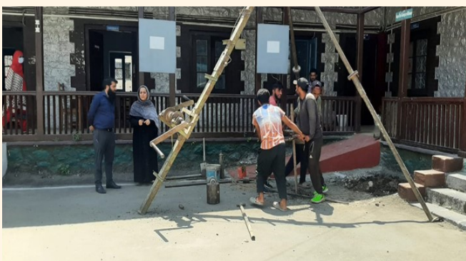
Soil Testing in Progress in connection with the construction of academic cum establishment Block.
